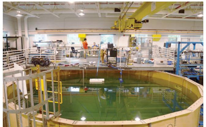
Fig. 5. Testing tank and loading platform. The tank is a 4.6-m (15-ft) tall, 8-m (26-ft) diameter, and  $250\text{-m}^3$  (65 000-gal) capacity cylindrical water reservoir. The platform spans on top of the tank. The six cameras for the motion capture system are installed at the bottom of the tank, fixing the field of view toward the area next to the platform.
