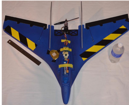
Fig. 2 Delta wing outfitted with an AMP board.
