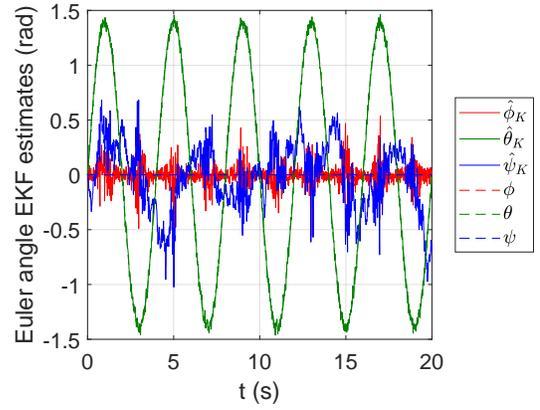
Fig. 4: Filtered estimation using an optimally tuned extended Kalman Filter (EKF). It can be seen that the EKF estimate  $\hat{\phi}_K$ ,  $\hat{\theta}_K$ , and  $\hat{\psi}_K$  has higher residual noise in comparison with figure 5, which can be traced to the linearization of the nonlinear attitude dynamics.
