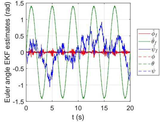
Fig. 5: Filtered estimation using equation (9). It can be seen that the proposed estimator yields more accurate estimates,  $\hat{\phi}_f$ ,  $\hat{\theta}_f$ , and  $\hat{\psi}_f$ , than the optimally tuned EKF (*cf* figure 4).
