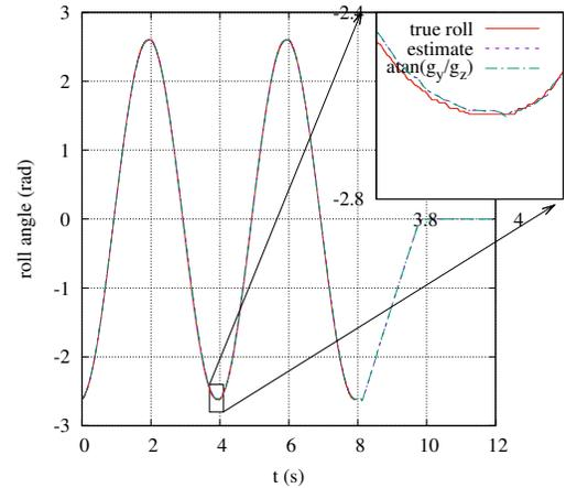
Fig. 2: Attitude estimation for a pure sinusoidal roll manoeuvre on a real system. The solid red line is the true roll angle returned by the encoder, and the dashed blue curve is the estimated roll angle. The small residual estimation errors can be mostly traced to alignment inaccuracies of the testbed. The vector measurements,  $g_y$  and  $g_z$ , are also included to show the instantaneous response from the measurement to the estimation.
