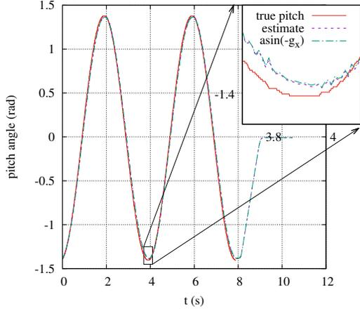
Fig. 3: Attitude estimation for a pure sinusoidal pitch manoeuvre on a real system. The solid red line is the true pitch angle returned by the encoder, and the dashed blue curve is the estimated pitch angle. The small residual estimation errors can be mostly traced to alignment inaccuracies of the testbed. The vector measurement,  $g_x$ , is also included to show the instantaneous response from the measurement to the estimation.
