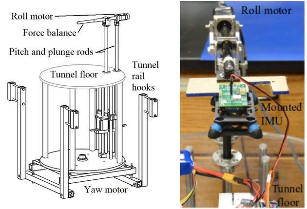
Fig. 1: On the left, a schematic of the 4 Degree of freedom Model Positioning System (MPS) described in [14]. The MPU9250 mounted on the PCB (green in the picture on the right) and being tested on the MPS.
