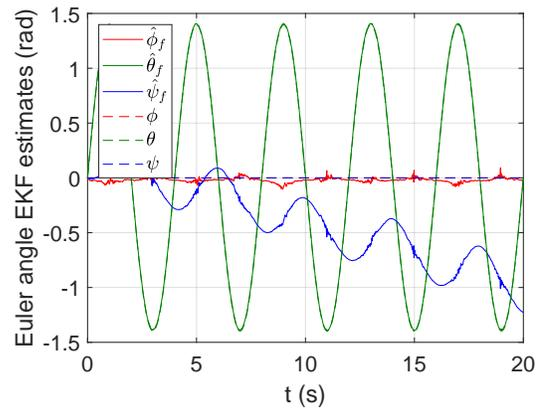
Fig. 6: Filtered attitude estimation in the presence of time-varying gyroscopic bias. Estimates  $\hat{\phi}_f$ ,  $\hat{\theta}_f$ , and  $\hat{\psi}_f$  of  $\phi$ ,  $\theta$ , and  $\psi$  are obtained using equation (14) and used for bias estimation (figure 7). Notice the steady yaw-drift with bias.
