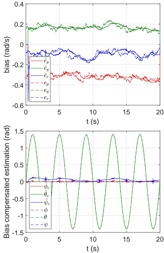
Fig. 7: Fail safe estimation of time-varying gyroscopic bias. A filtered attitude estimate is obtained using equation (14) (cf figure 6). The attitude correction from the integrated attitude estimate to the filtered estimate is inverted to obtain the bias error under persistent excitation (top). The filtered attitude is then corrected further to obtain compensated estimate,  $\hat{\phi}_c$ ,  $\hat{\theta}_c$ , and  $\hat{\psi}_c$ , that gets rid of the low frequency errors in the bias (bottom).
