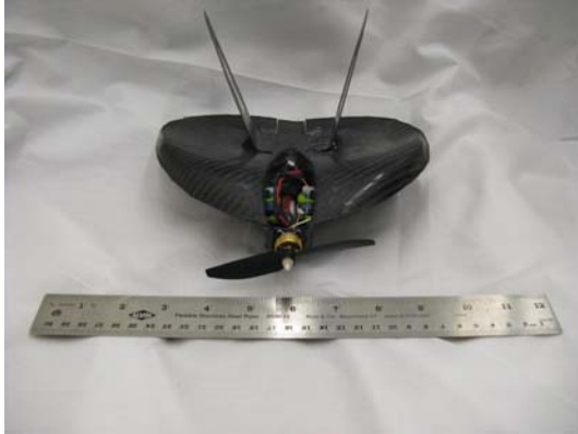
Figure 1. PIPER MAV developed by the group; photo from December 2008.
