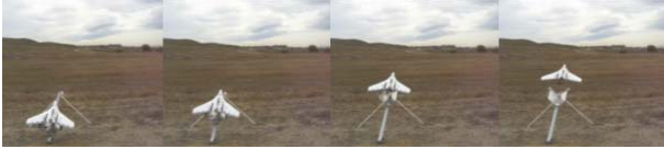
Figure 4. Plane-A-Pult Automatic Aircraft Launcher performing a fully autonomous launch.
