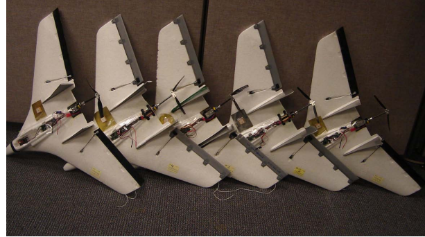
Figure 5. Our first flock of 5 MAVs. The design of each MAV is relatively simple, so scaling to produce larger flocks can be quickly achieved.
