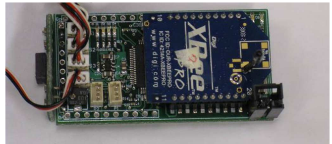
Fig. 16. CUPIC autopilot weighs 19 grams and is 6 cm × 3 cm × 1.4 cm in dimensions.
