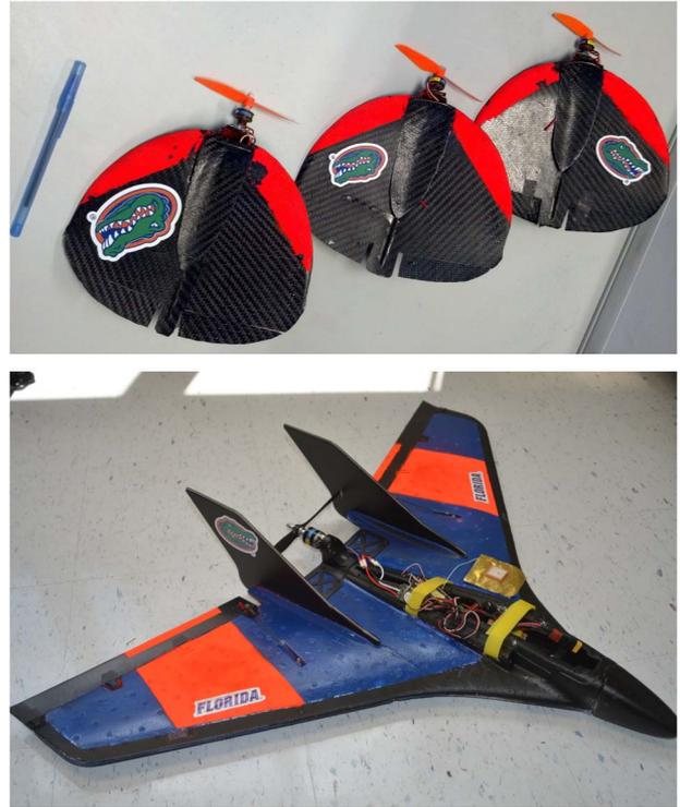
Fig. 1. Two examples of autonomous micro and miniature aerial vehicles in our group. Top: 60-g MAV with the wing span of 8 in and a payload capacity of 20 g [6], [7]. Bottom: 250-g miniature aerial vehicle with the wing span of 2 ft and a payload capacity of 100 g [5], [8]. All vehicles are equipped with GPS, radio, transmitter, pressure, temperature and humidity sensors, inertial measurement unit (IMU), etc.
