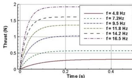
Along with a minimal rise time, the VRT is also immune to a thrust lag seen in tunnel thrusters (McLean, 1991), where thrust continues to be exerted on the vehicle after the thruster has been terminated.
