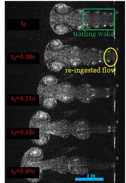
impulse (with respect to the momentum impulse,  $I_{slug}$ ), it is only observed in low actuation frequencies, which are coupled with low thrust output. Often vehicle mission scenarios will necessitate a large magnitude thrust output (higher actuation frequencies), where the overpressure is cancelled out, and the slug model provides an accurate thrust measurement.
