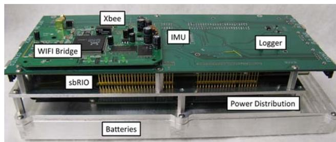
ics located in the center section, where everything except the motor controllers and user interface is located.
