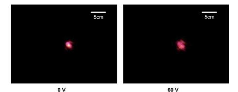
Fig. 14. Images of a laser beam passing through the microlens with 0 V and 60 V applied.
