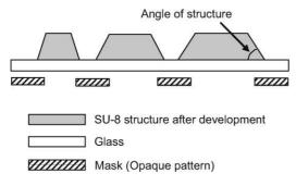
Fig. 10. Control of angle of slanted SU-8 structure (not to scale).
