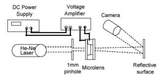
Fig. 13. Schematic of experiment setup.
