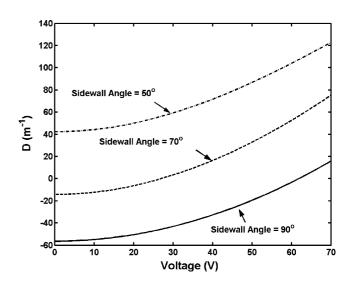
Fig. 9. Optical power of microlens as a function of voltage for sidewall angles of  $50^\circ$ ,  $70^\circ$ , and  $90^\circ$ .
