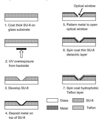
Fig. 6. Fabrication process of bottom substrate structure.
