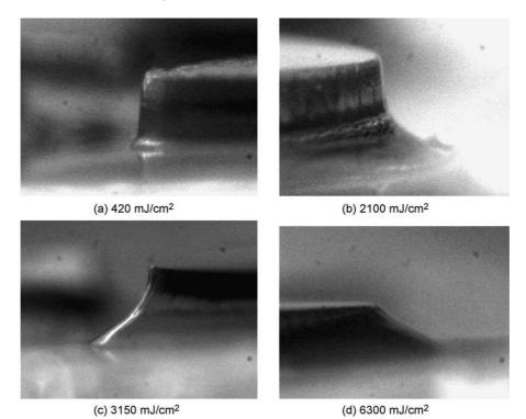
Fig. 5. Profile of SU-8 sidewall with different exposure dosages.
