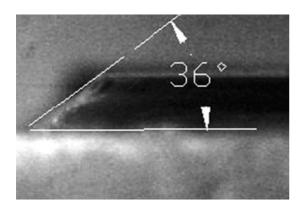
Fig. 8. Angle of sidewall of the SU-8 structure.
