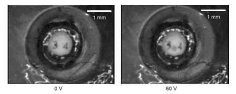
Fig. 12. Images (numbers '3' and '4') captured at 0 V and 60 V applied to the microlens.
