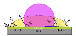
Fig. 1. Schematic view of principle of EWOD.
