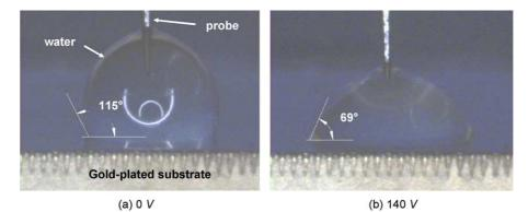
Fig. 2. Change of the contact angle of water on SU-8 coated substrate.
