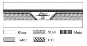
Fig. 4. Schematic view of the variable focus microlens.
