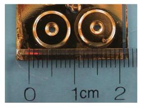
Fig. 7. Tapered SU-8 structure (top view).
