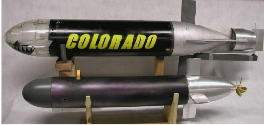
Figure 7: UUV test beds at the University of Colorado. (Top) HydroBuff: A remotely controlled unmanned underwater vehicle [6]. (Bottom) RAV: An RC UUV capable of housing 4 pulsatile jet actuators [5].
