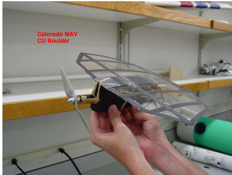
Figure 1. Membrane wing MAV under development at the University of Colorado. Wingspan is 30 cm and mass is 170 g.
