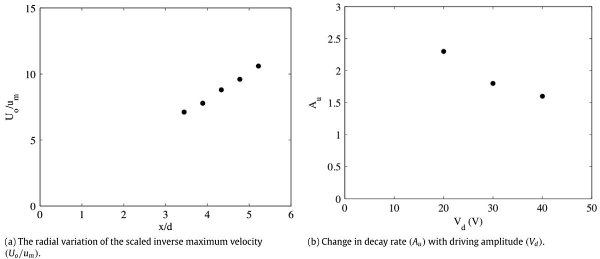
Fig. 10. Decay of the maximum centerline velocity.
