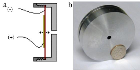
**Fig. 6.** A round synthetic jet actuator: (a) a schematic (b) an actuator alongside a dime provided for scale.
