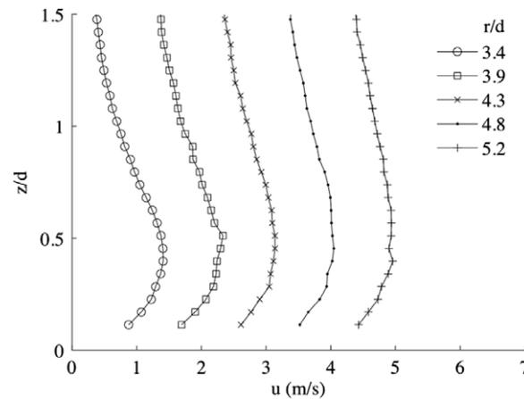
Fig. 9. The evolution of the mean velocity profiles in the radial direction. The velocities are displaced by 1 m/s successively starting at  $r/d = 3.9$ .
