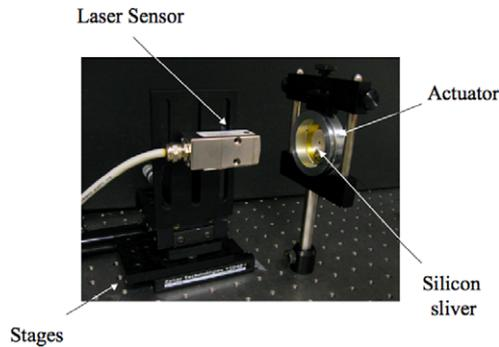
Fig. 7. The experimental setup used to obtain the deflection of the oscillating diaphragm.
