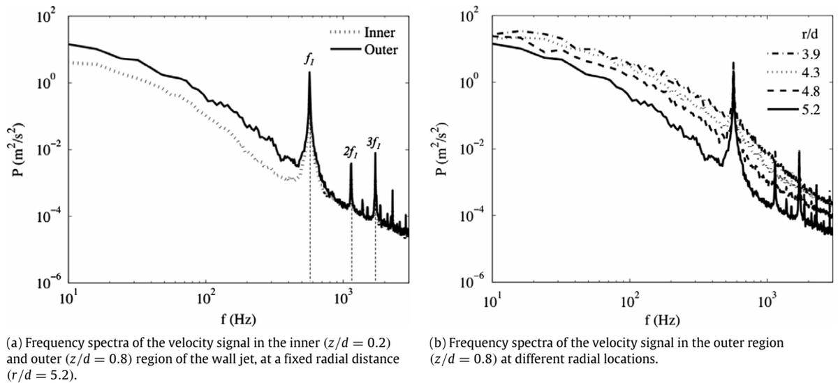
Fig. 13. Frequency spectra in the wall jet region.
