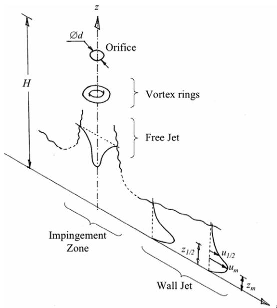
**Fig. 2.** Schematic of the evolution of the flow due to the normal impingement of a round synthetic jet upon a wall. Shown, are vortex rings in the near field of the orifice, and mean velocity profiles of both, free and wall jets in the far field.
