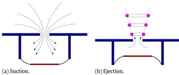
**Fig. 1.** Schematic of the synthetic jet operation displaying the suction and ejection strokes.
