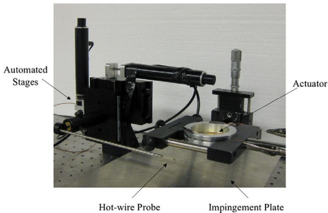
**Fig. 5.** The experimental setup used to measure the velocity field in the radial wall jet.
