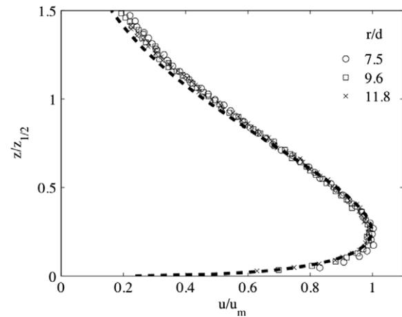
Fig. 8. The normalized mean velocity profile of a wall jet induced by the normal impingement of a continuous jet. The dashed line represents a semi-empirical turbulent solution.
