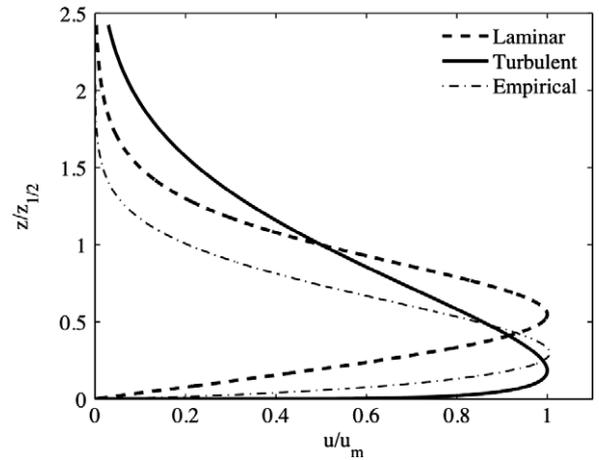
Fig. 3. Representative velocity profiles of the closed form laminar, semi-empirical turbulent, and empirical wall jet solutions. The dashed line represents the classic laminar wall jet solution, the solid line shows a turbulent jet solution for  $\alpha = 1.4$ , while the dash-dot line shows an intermediate profile that is later seen to represent the synthetic wall jet for the parameters employed.
