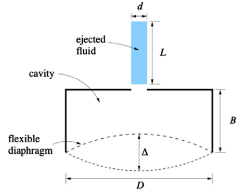
Fig. 4. Schematic of the actuator model, where the volume of fluid displaced by the diaphragm is ejected through the orifice in the form of a slug.
