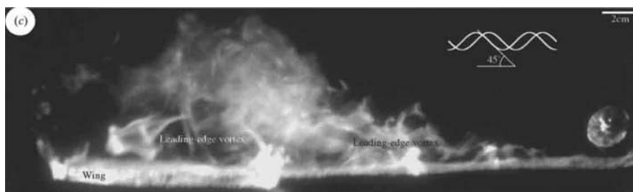
Fig. 1 Visualization of a helical leading edge vortex in a hovering hawkmoth. The image also shows an increase in LEV size with distance from the base of the wing. Figure adapted from van den Berg and Ellington (1997b). The view is parallel to the wing chord.
