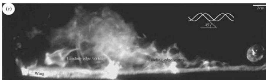
Fig. 1 Visualization of a helical leading edge vortex in a hovering hawkmoth. The image also shows an increase in LEV size with distance from the base of the wing. Figure adapted from van den Berg and Ellington (1997b)
