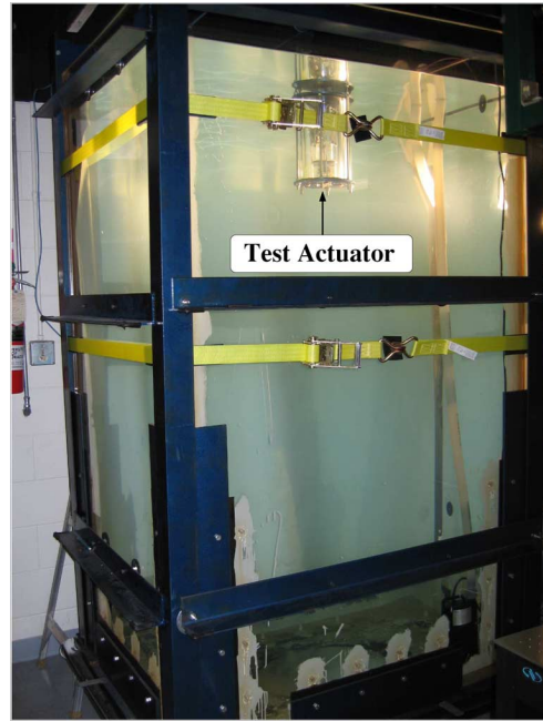
Fig. 5. Actuator testing tank.
