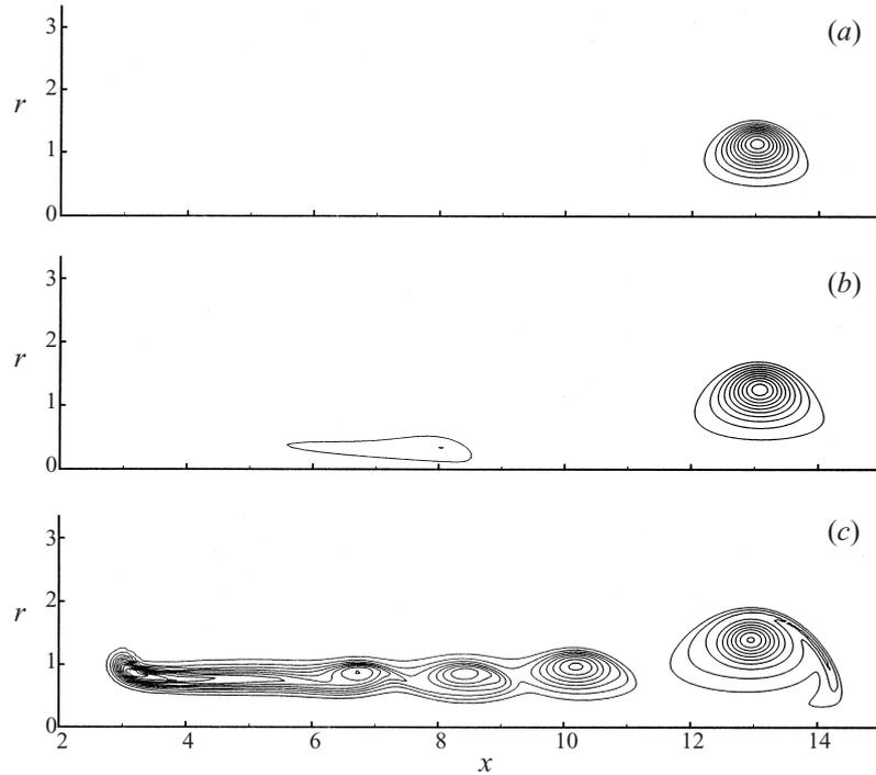
FIGURE 3. Vortex ring formation with different forcing times. (a)  $TC/R^2 = 4.05$  (Case 2), contour levels (min = 0.002, max = 0.02, increment = 0.002); (b)  $TC/R^2 = 25.3$  (Case 5), contour levels (min = 0.0023, max = 0.0333, increment = 0.0031); (c)  $TC/R^2 = 77.5$  (Case 7), contour levels (min = 0.0023, max = 0.0333, increment = 0.0031).
