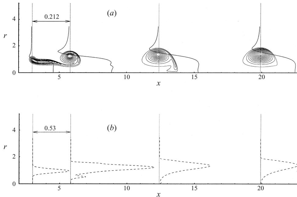
FIGURE 6. Long-duration forcing. (a) Non-dimensional vorticity contours ( $\omega R^2/C$ ) and axial velocity ( $uR/C$ ) profiles, and (b) vorticity profiles at non-dimensional times  $tC/R^2 = 46.8, 122.7,$  and  $217.6$ : axial velocity (—) and azimuthal vorticity (---). Axial velocity and vorticity distributions at the axial centre of the forcing region at  $tC/R^2 = 46.8$  is also plotted. The scales for velocity and vorticity profiles are shown.
