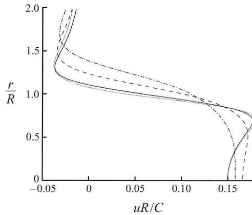
FIGURE 5. Velocity profile at time  $tU_{tr}/D = 9.11$  for forces with different values of  $\alpha_r/R$ .  $\alpha_r/R = 0.6$ , Case 16 (— · —);  $\alpha_r/R = 0.4$ , Case 15 (---);  $\alpha_r/R = 0.2$ , Case 5 (—);  $\alpha_r/R = 0.1$ , Case 14 (·····).
