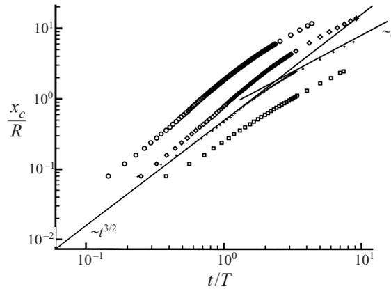
FIGURE 1. Distance of the vortex centre from the forcing location for different duration of forces. Case 1,  $TC/R^2 = 1.58$  ( $\square$ ); Case 2,  $TC/R^2 = 4.05$  ( $+$ ); Case 3,  $TC/R^2 = 9.11$  ( $\diamond$ ); Case 4,  $TC/R^2 = 25.3$  ( $\circ$ ). Other parameters associated with the cases are given in table 1.
