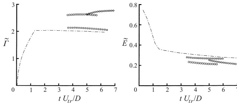
FIGURE 8. Vortex rings generated with time-varying forcing. Case 3 (— · —); Case 5 ( $\square$ ); Case 17, variable amplitude ( $\circ$ ); Case 18, variable radius ( $\diamond$ ).
