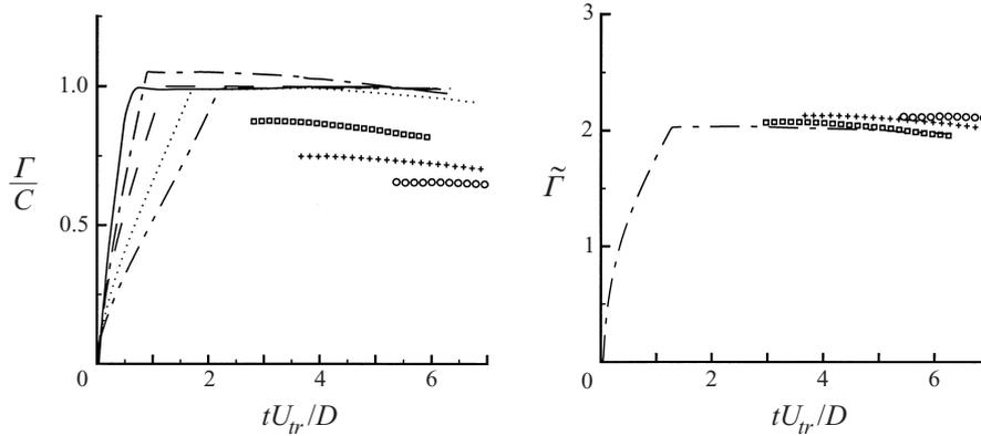
FIGURE 4. Vortex rings with different forcing duration. (a) Circulation normalized by forcing amplitude,  $\Gamma/C$ . (b) Normalized circulation,  $\tilde{\Gamma}$ . The lines correspond to total circulation, while the symbols correspond to circulation of the leading vortex ring.  $TC/R^2 = 4.05$ , Case 2 (—);  $TC/R^2 = 9.11$ , Case 3 (— · —);  $TC/R^2 = 14.2$ , Case 4 (--- and  $\square$ );  $TC/R^2 = 25.3$ , Case 5 (····· and +);  $TC/R^2 = 39.5$ , Case 6 (— · — and  $\circ$ ).
