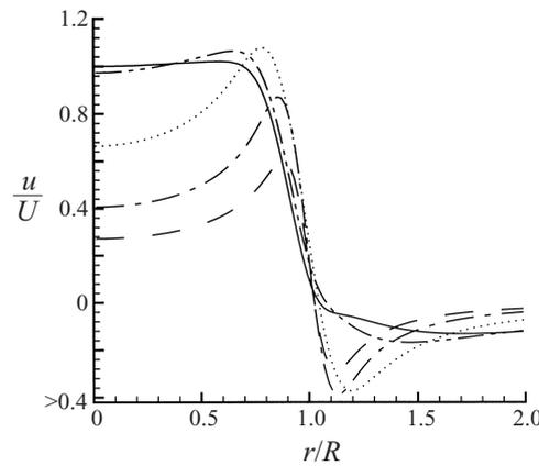
FIGURE 2. Axial velocity at the centre of the forcing region for Case 14 of table 1.  $tC/R^2 = 8.86$  (----);  $tC/R^2 = 11.4$  (-.-.-);  $tC/R^2 = 16.4$  (.....);  $tC/R^2 = 26.6$  (— · — · —);  $tC/R^2 = 31.6$  (—). The velocity is normalized with the maximum axial velocity at time  $tC/R^2 = 31.6$ .
