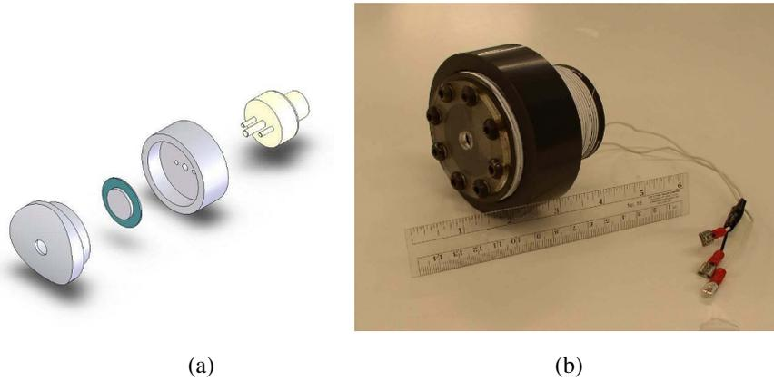
Fig. 4. CU Boulder Synthetic jet prototype [13], [14]: (a) Plunger and solenoid assembly. (b) Actual fabrication of the synthetic jet actuator.
