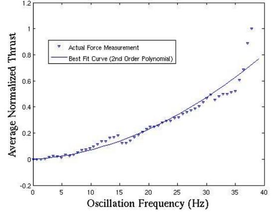
Fig. 10. Actuator thrust response (symbols) and fitted curve (solid line) in the frequency domain for  $L/D = 3.93$ .
