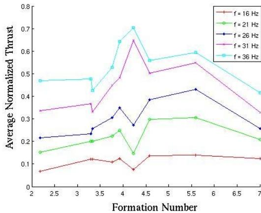
Fig. 12. Averaged normalized actuator thrust response in formation number domain.
