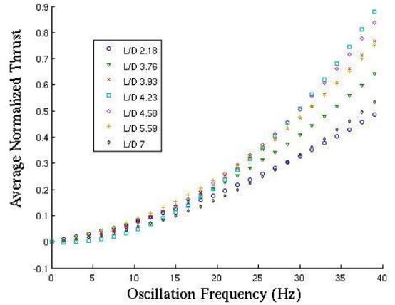
Fig. 11. Curve fitted actuator thrust response in the frequency domain for various formation numbers.
