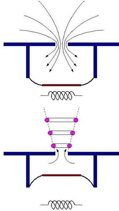
Fig. 3. Synthetic jet actuator concept: (Top) Fluid entrainment; (Bottom) vortex ring formation.
