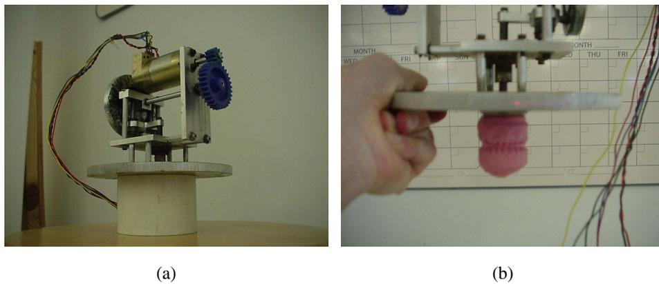
Fig. 7. Mechanical plunger setup (a) motor, gear and cam assembly. (b) Piston/plunger inside the cavity.
