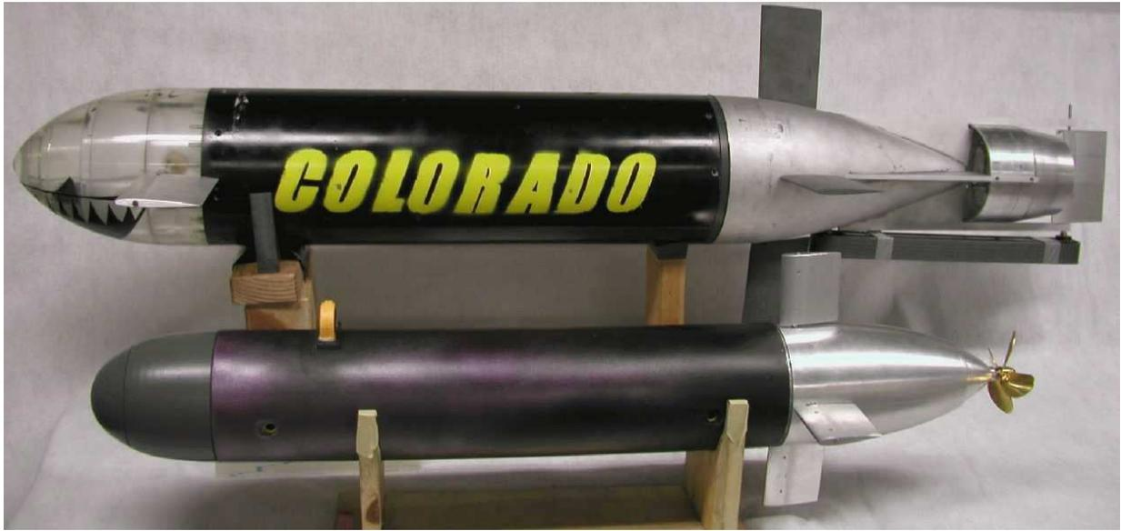
Fig. 5. University of Colorado Test Beds. The smaller vehicle is equipped with 4 synthetic jet actuators.
